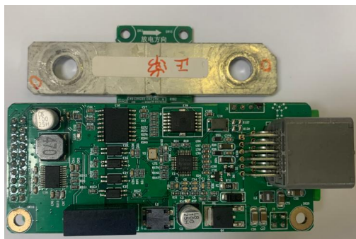
BMS high-voltage control board
